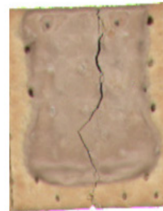
Cracked (filtered color blob analysis)
