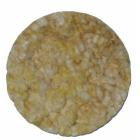
**True color calculations**, on both the top and bottom surface of the product, are measured in various units such as L\*a\*b\* and BCU.
