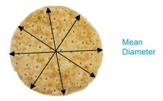
**Two dimensional calculations** are based on an accurately defined perimeter, which is imaged by both overhead cameras. 2-D measurement accuracy is ±0.5mm. Length, Width, Maximum Diameter, Minimum Diameter, Diameter Range, and Surface Area are other common measurements applied to pancakes, thins, and other similar products.
