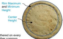
**Profile height calculations** are based on hundreds of individual height values gathered on every product, which leads to a measurement accuracy of ±0.5mm. Mean Height is another common measurement applied to pizza crust, flatbread, and other similar products.
