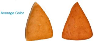
**True color calculations** are measured in various units such as L\*a\*b\* and BCU, which <u>quantify small variations of bake color</u>.
