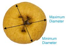
**Two dimensional calculations** are based on an accurately defined perimeter, which is imaged by both overhead cameras. 2-D measurement accuracy is ±0.5mm. Mean Diameter, Roundness, Surface Area, and Volume are other common measurements applied to donuts.
