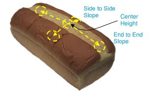
**Profile height calculations** are based on hundreds of individual height values gathered on every product, which leads to a measurement accuracy of ±0.5mm. Mean Height is another common measurement applied to bagels.
