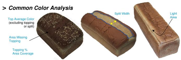
**True color calculations**, on both the top and bottom surface of the product, are measured in various units such as L\*a\*b\* and BCU. Bottom color and Dark Area are other common color measurement applied to bread loaves
