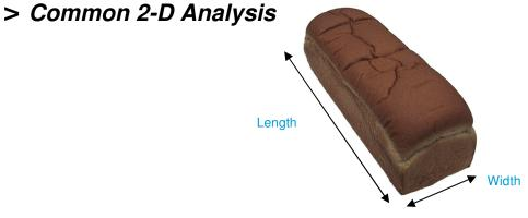
**Two dimensional calculations** are based on an accurately defined perimeter, which is imaged by both overhead cameras. 2-D measurement accuracy is ±0.5mm. Surface Area and Volume are other common dimensional measurements applied to bread loaves.
